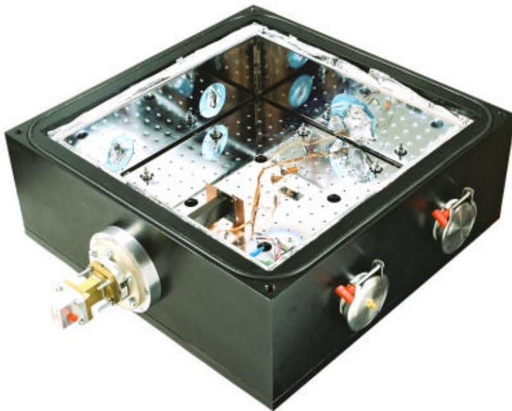
Test Dewar: Cover removed
